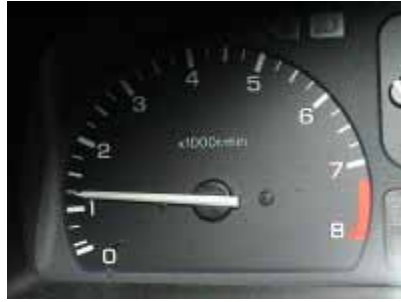
Figure 3.2: Revolution meter indicating the actual engine speed
