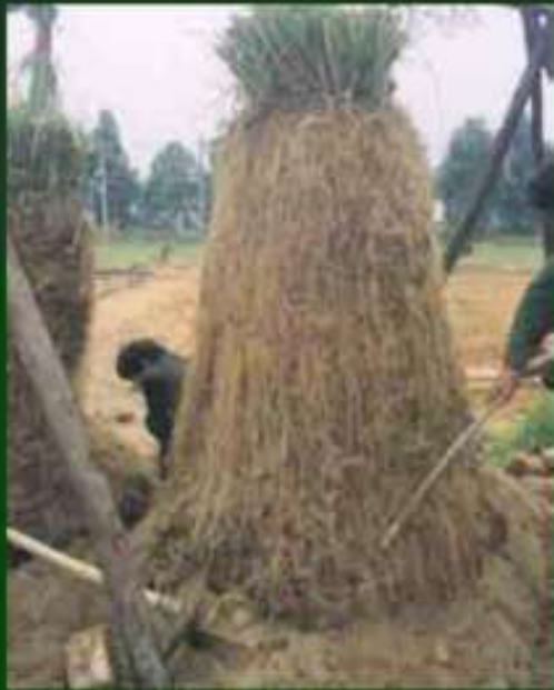
China - excavated root. Average tensile root strength 75 MPa
