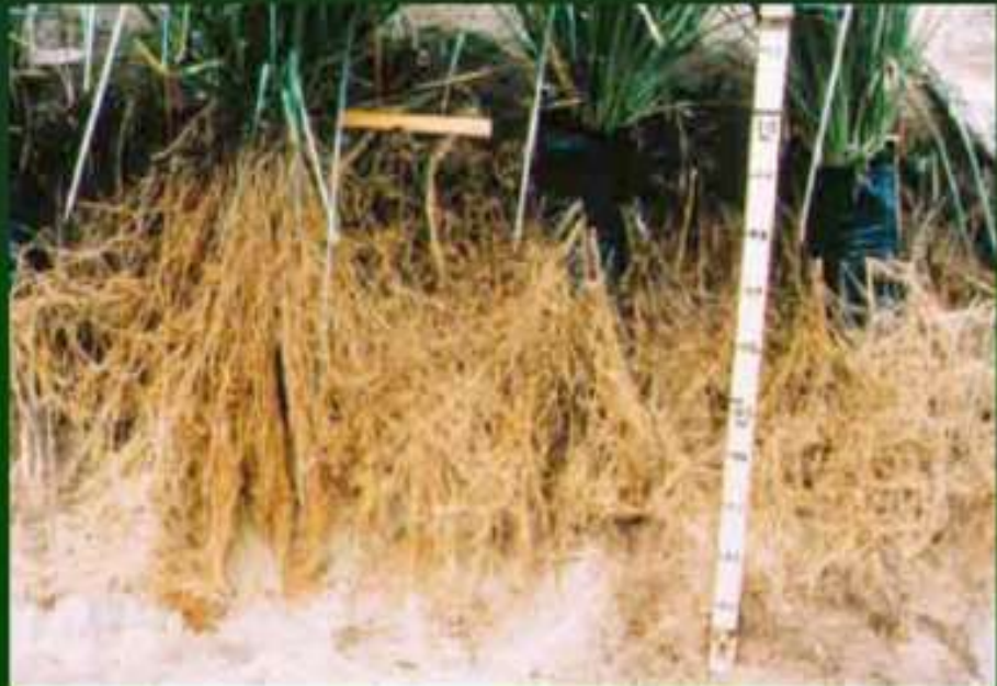
Malaysia - longitudinal section through hedge note the root mass in the top meter of the soil profile. This type of root mass will improve soil shear strength by up to 39%
