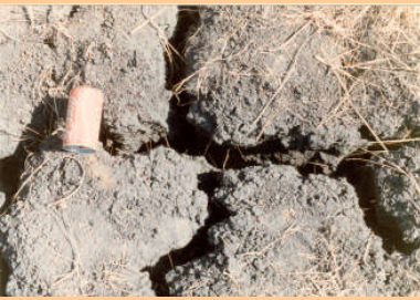
Expansive “black cotton” soil exhibiting wide-spaced shrinkage
