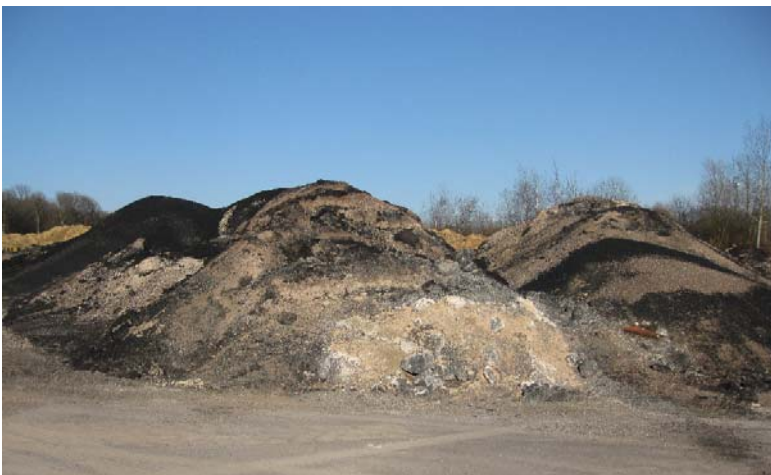
Figure 9: Wasted asphalt and aggregates next to a drum mix plant)
