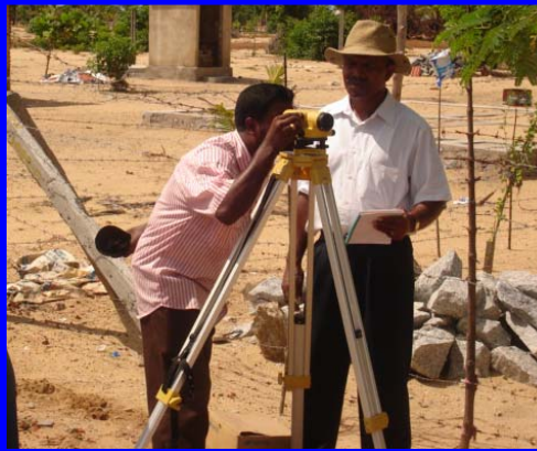
Taking of levels for compilation of design
