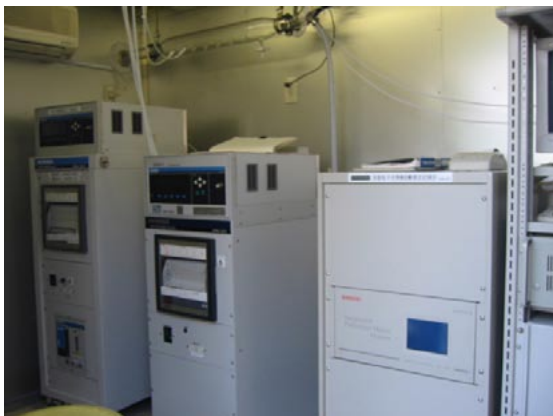
Fig. 19.15 Air quality analysing equipment for NO x , CO, and PM.
