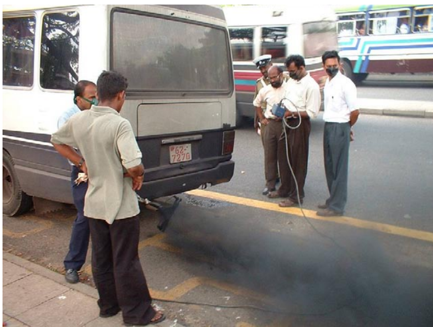
Fig. 19.18 Random, on-street spot monitoring of vehicles can be an effective way of ensuring regulatory norms are met in practice.
