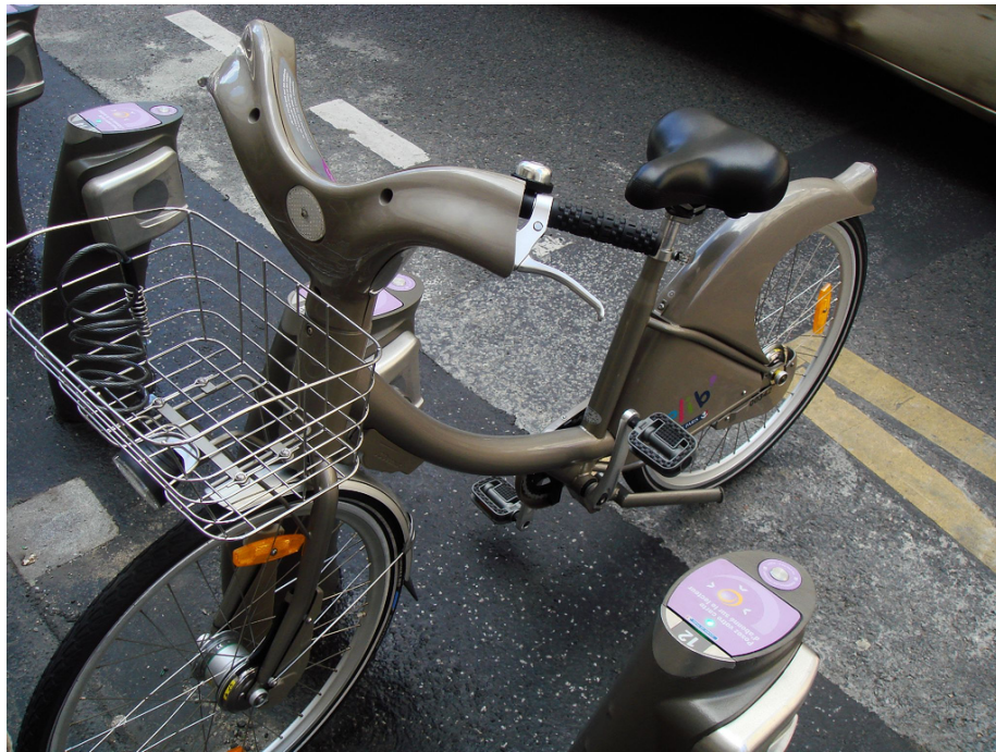
Figure 10 Vélib bicycles have an auxiliary cable lock, seen here inside the basket, that allows users to lock the bicycle temporarily between stations
