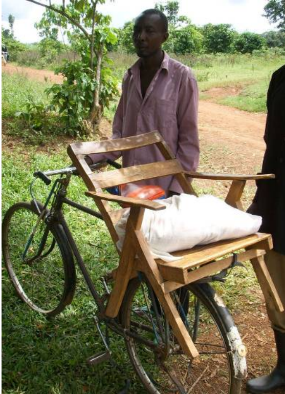
Figure 3: Bicycle with a chair on the carrier to transport patients
