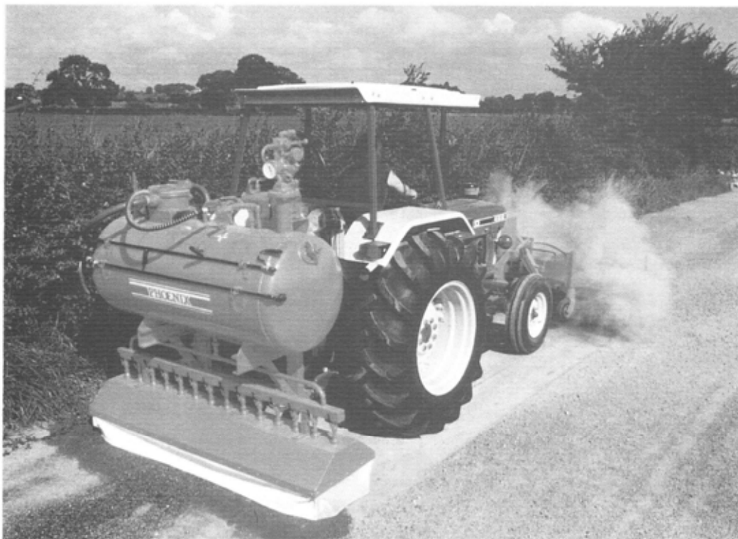
Figure 20 - Tractor Fitted with Hydraulically Driven Road Sweeper and 550 Litre Bitumen Emulsion Sprayer
