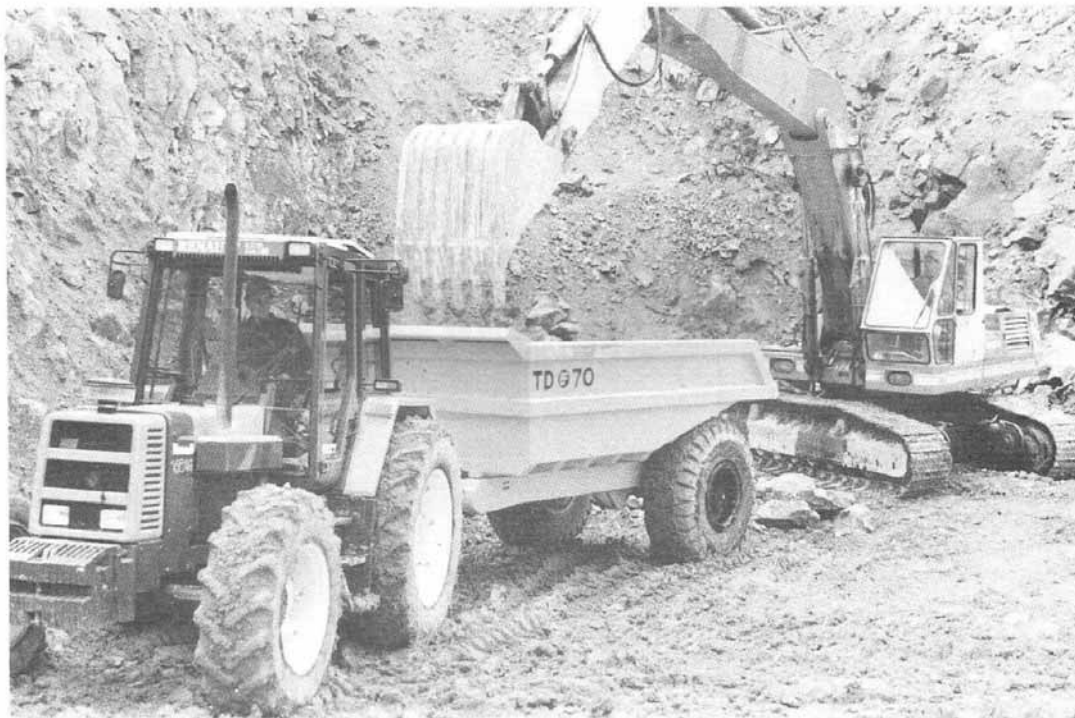
Figure 9 - 3 Cubic Metre Gravel Haulage Trailer for Labour Loading and Unloading
