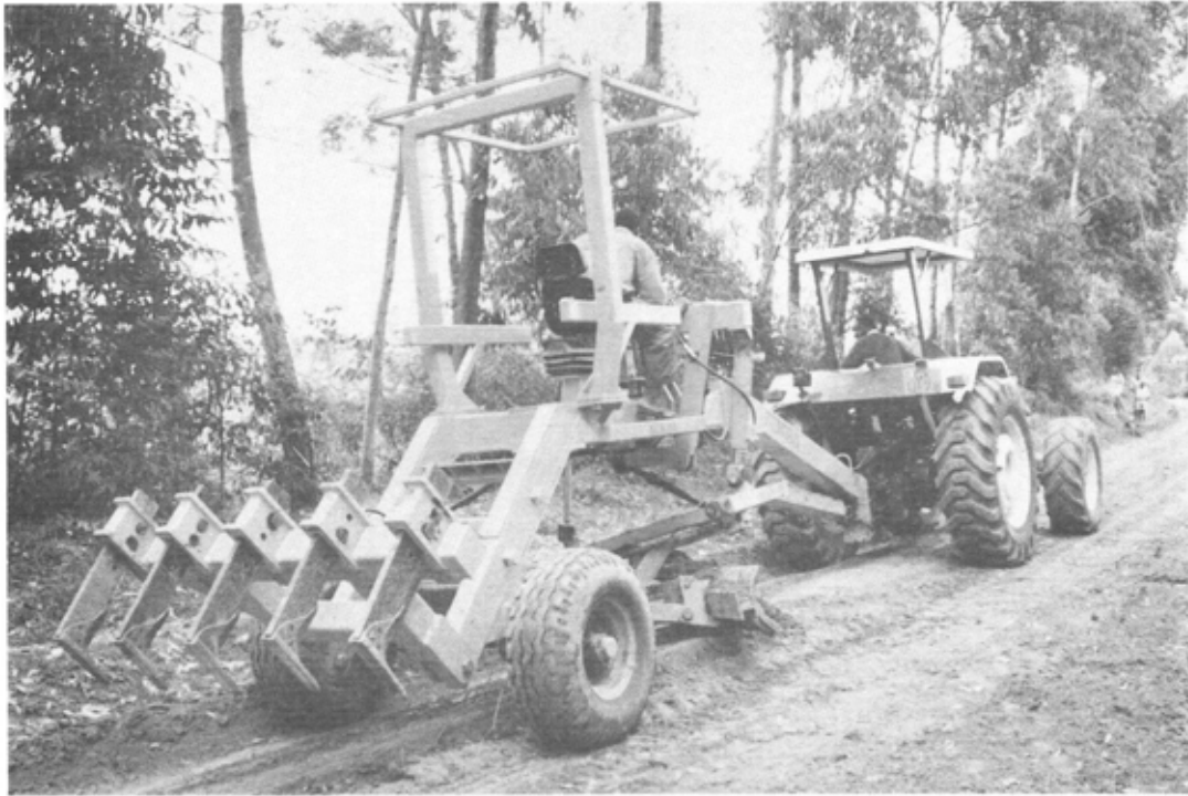
Figure 15 - 4/5 Tonne Heavy Towed Grader with Ripper Attachment
