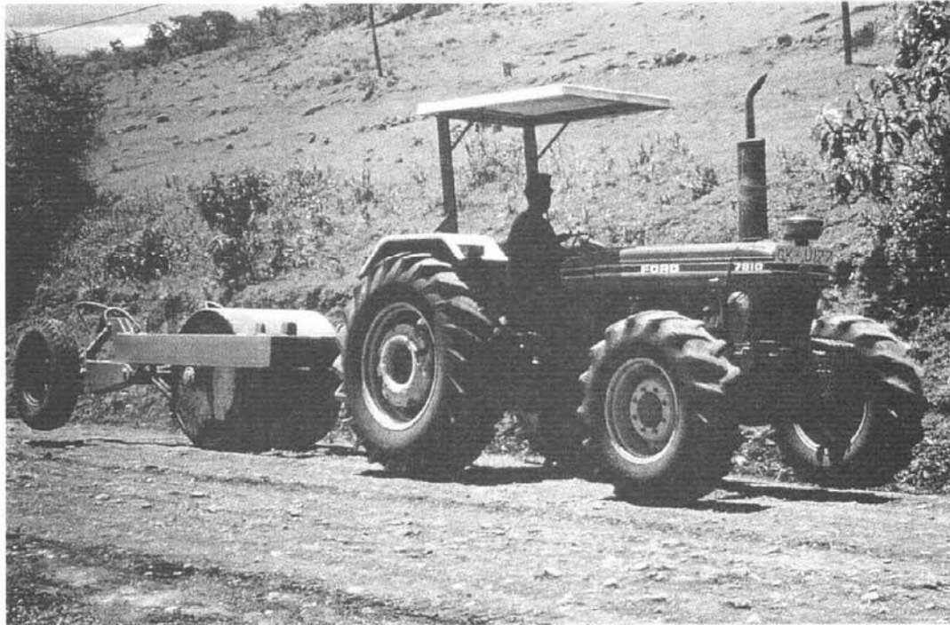
Figure 17 - 5 Tonne Towed Deadweight Roller with Transport Wheels
