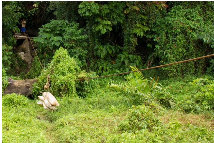
The Flying Fox method of transporting guano from the cave to the drying location
