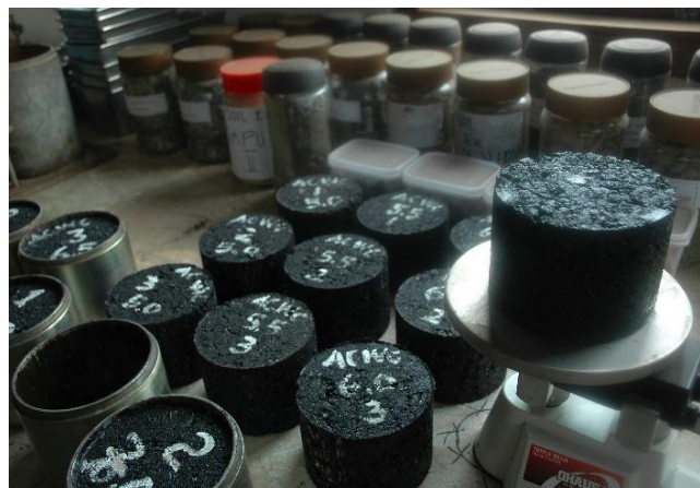
Asphalt plugs are removed from the road for examination.
