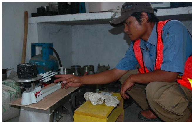
A laboratory worker weighs the asphalt before checking its density and stability.
