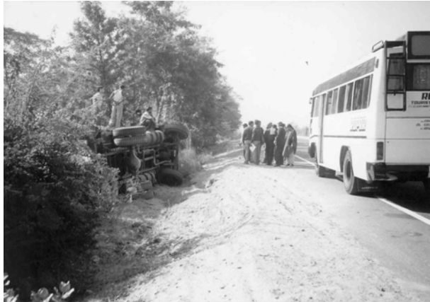
Figure 10. Truck rollover on highways on embankments without guardrails.
